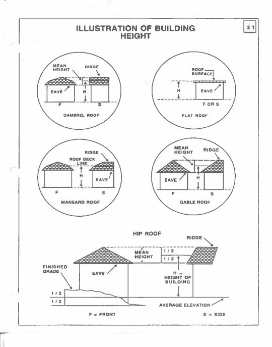
The above illustrates the method of calculation of Building Height for various types of roof forms. It also illustrates the method of calculation of the average elevation of the finished grade within 10 feet of the walls of the building.
